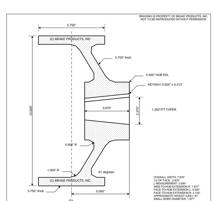
TOLERANCES: WHEEL DIAMETER: +0.005"/-0.000" BORE TAPER: +0.000"/-0.003"
